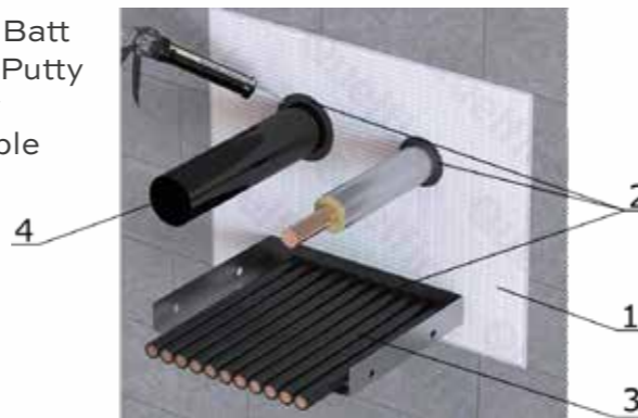
Figure 2. Smart Fire Batt with combustible pipes and cable tray (sealed with Smart Fire Putty)
